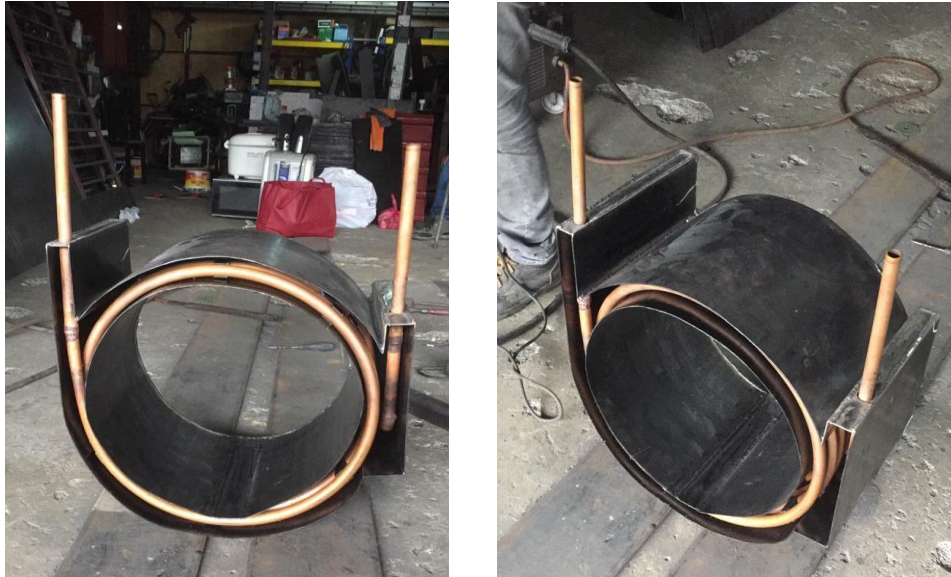
Figure 49: Front view and top view of fully welded tank
